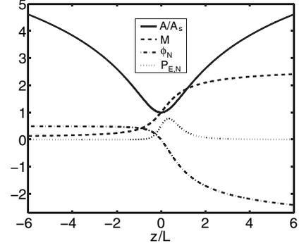
FIG. 2. The DL in a plasma flow along a converging-diverging magnetic field (similar to [7]). Shown are the profiles of the normalized (as defined in the text) cross section  $A/A_s$ , Mach number  $M$ , potential  $\phi_N$ , and electrostatic pressure  $P_{E,N}$ .
